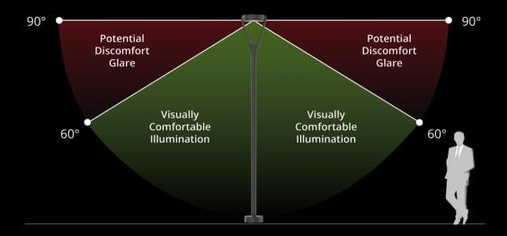
Light exiting the luminaire at angles that typically cause visual discomfort is minimized, without compromising performance. BUG ratings for glare of G1 or G2 create an environment suitable for almost any application.
