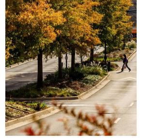
of plant basin is a bioswale. A bioswale is a linear channel that is designed to slow and filter stormwater as well as divert the runoff water from traveling directly into nearby rivers. This type of channel works very well to combat the greater quantities of stormwater, or floods, that occur because of impervious surfaces such as asphalt. The bioswales are also constructed of mostly native plants, which provide habitats and food for local species.
