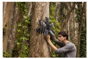
cellular energy. The devices are placed high in the tree canopy of the rainforest and can detect chainsaw noises up to a mile away. When the device detects chainsaw frequencies, a text alert is sent to authorities so that they can appropriately handle the situation and work to save our rainforests! Click the button below to learn more about Topher, his device, and the *Rainforest Connection*.
