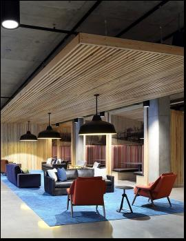
Our Oversized Shade OSAB42, 42 inches in diameter, was selected for the soft seating social workspace areas to fill the overhead space. A domed, wider distribution lens on the dimmable LED module, provides even, energy efficient illumination.
